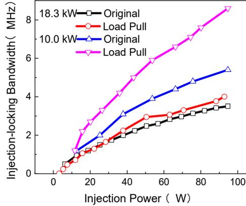
Fig. 3. The injection locked bandwidth with various injection ratios at different state.
