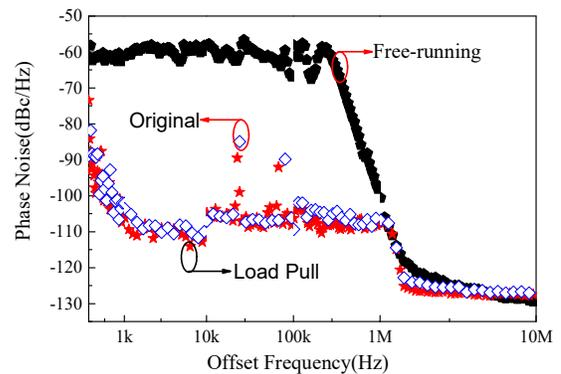
Fig. 4. The phase noise of the magnetron.
